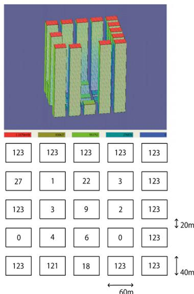
Figure 4 Optimisation of tower height within a regular grid for solar irradiation utilisation
