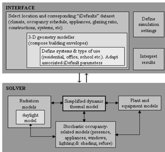
Fig 3. Conceptual structure of SUNtool
